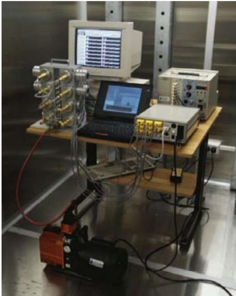
FIG. 1. Radon progeny particle size spectrometer
