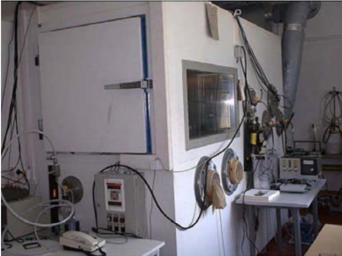
FIG .1. The radon chamber at CLOR
