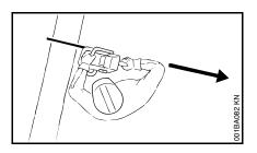
Position the chainsaw in such a way that your body is clear of the cutting attachment whenever the engine is running. Stand to the left of cut while bucking.
