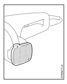
Cooling air flows to the motor through the slots in the commutator cover.
