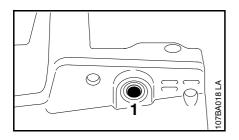
The overload circuit breaker cuts off the power supply to the saw in the event of mechanical overload due to, e.g.
