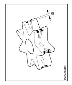
Replace the chain sprocket
