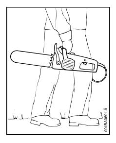
By hand: When carrying the chain saw by hand, it must be switched off and the saw held in the proper position, i.e. it should be gripped by the front handle. The chain guard must be fitted, even when carrying the saw only a short distance, and the guide bar must point backwards, away from the direction in which you are going.
