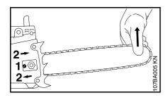
Retensioning during cutting work:
