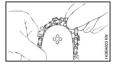
Turn the guide bar so that the chain cutting edges on the top of the bar point toward the bar nose (see illustration).
