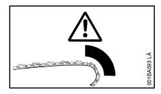
the powerful force used to cut wood can be reversed (and work against the operator). If the rotating chain is suddenly stopped by contact with any solid object like a log or branch or is pinched, the reactive forces may occur instantly. These reactive forces may result in loss of control which may, in turn, cause serious or fatal injury. An understanding of the causes of these reactive forces may help you avoid loss of control.
